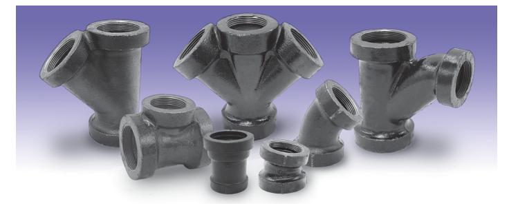
Anvil drainage fittings have sufficient sweep to allow free unobstructed flow. They are made with a shoulder of the same diameter as the inside of the pipe, in accordance with ASME B16.12, Type 1. Thus, continuous passage is created when the pipe is screwed to the shoulder, leaving no place for solid matter to collect and clog in the pipe. Drainage fittings with 90° bends are normally provided tapped with pitch of 1/4 inch to the foot in accordance with ASME B16.12.
